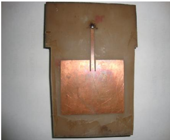
Fig1. Design of rectangular microstrip patch antenna
