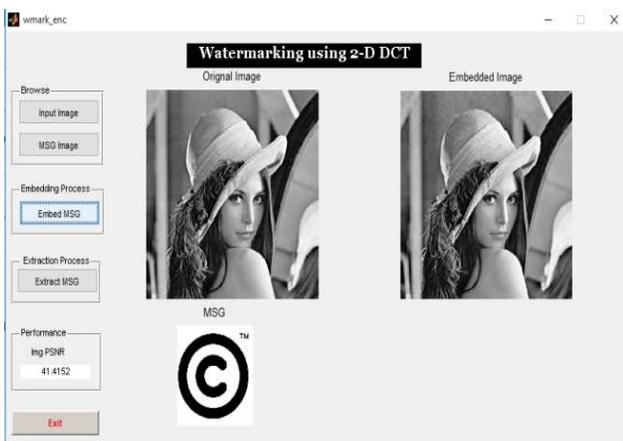
Figure 5: Embedded watermark image on original image using GUI
